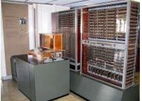
An early electromechanical programmable computer, the  $\mathbb{Z}_3$ , included floatingpoint arithmetic (replica on display at <u>Deutsches Museum</u> in <u>Munich</u>).
